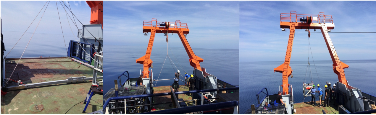
Fig. 7: Deployment of the MARTEMIS system on R/V Poseidon (pictures taken during cruise POS483).
