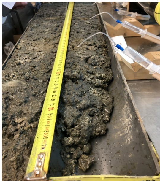
Fig. 27: Pore fluid sampling in POS524/01GC using Rhizons CSS with 4cm porous polymer tubes (photo by Shuangmin Duan)
