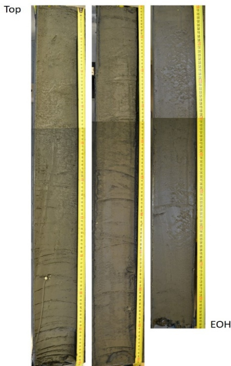
Fig. 29: Sediment core 04GC, collected 1km west of the main hydrothermal mound. is characterized by homogeneous greenish grey clay with strong smell of H 2 S.
